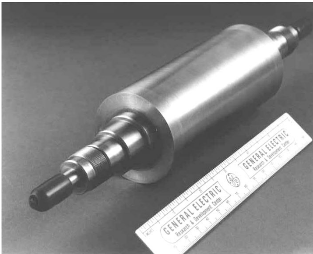
Fig. 3. Photograph of one of the completed preprototype induction motor rotors.
