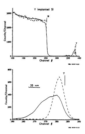
Fig. 2 Rutherford Backscattering spectra for Y into Si. The dashed curve is from the sample without pulse biasing and the solid curve from that with pulse biasing. The depth of implantation is approximately 500 A and the dose is  $1 \times 10^{16}$  cm<sup>-2</sup>. The second curve shows the detail of the Y distribution.
