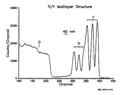
Fig. 3 Rutherford Backscattering spectra for a Ti-Y multilayer structure on Si with ion beam mixing at the first Si-Y and the final Ti-Y interfaces.
