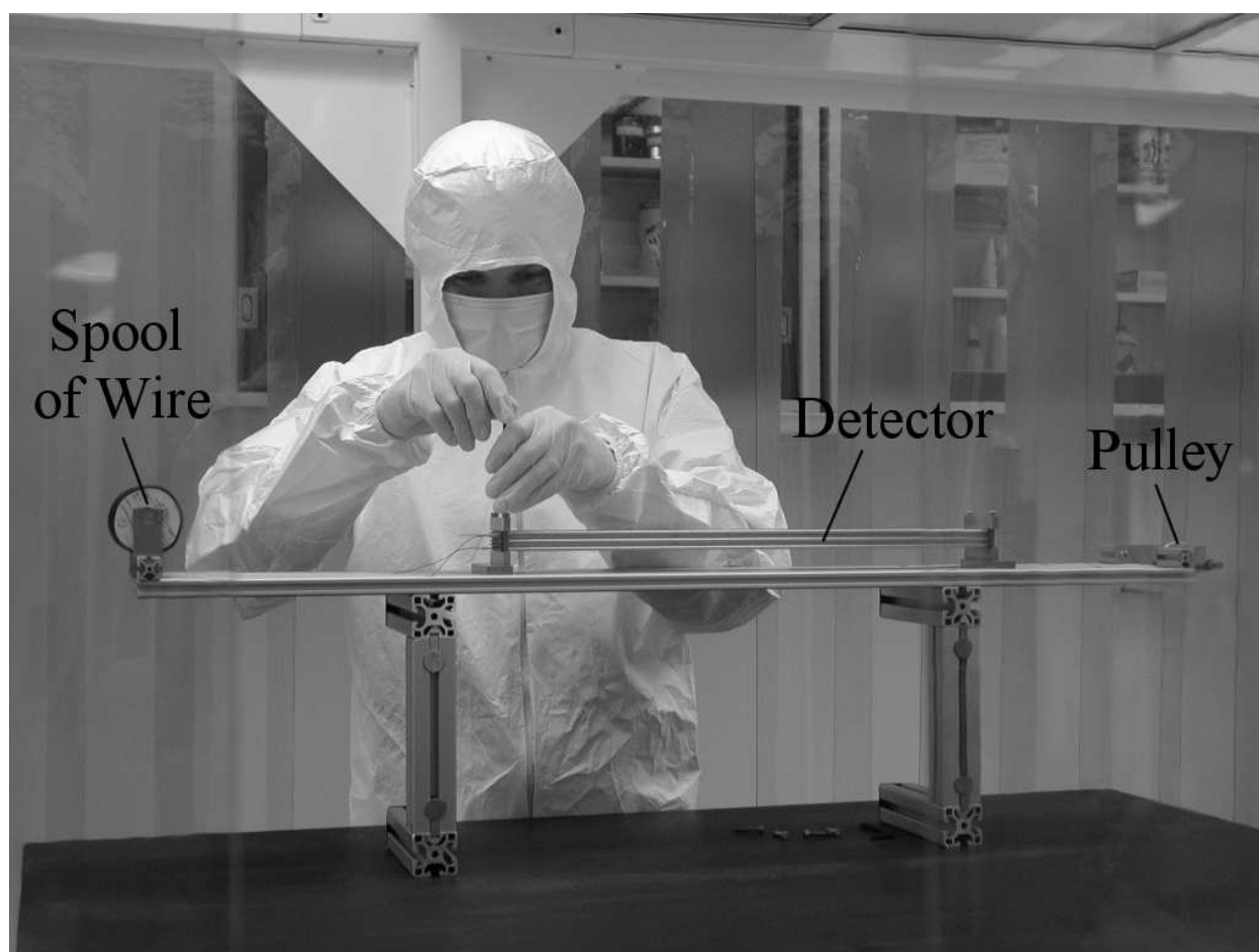
Figure 6: Fixture used for wiring straw detectors located in a class 100 clean room.
