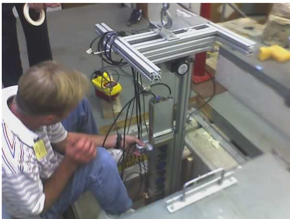
Figure 8: The prototype detector shown as it is lowered inside the cave that contains the neutron beam. A collimator with the letters “PROPORTIONAL TECH.” is attached on the front face of the detector.
