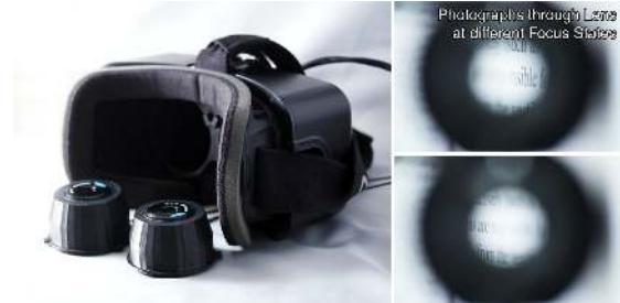
Figure 3. Photograph of HMD prototype and focus-tunable lens.
