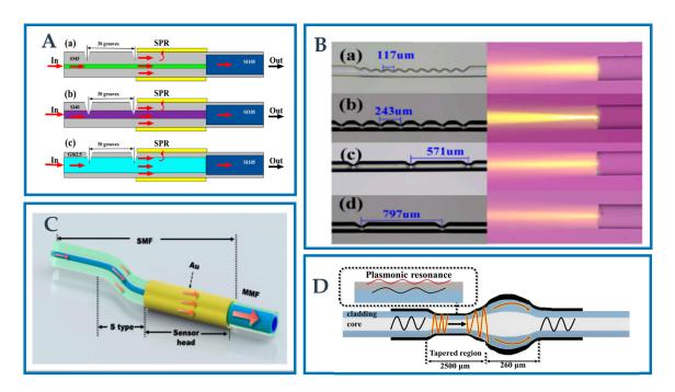
**Figure 9.** (**A**). Sensing schematic of V-groove-SMF structure (**a**–**c**). Reprinted with permission from Optics Communications, Copyright 2023, Elsevier [126]; (**B**). Schematic diagram of multi-V-groove structure (**a**–**d**). Reprinted with permission from Optics Communications, Copyright 2023, Elsevier [126]; (**C**). Schematic diagram and microscopic morphology S-shaped based SMF-MMF structure. Refer to [127]; (**D**). Schematic diagram of downward taper structure. Refer to [128].
