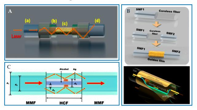
**Figure 6.** (**A**). The schematic of the sensor probe and each section of the probe: (**a**) single-mode fiber, (**b**) capillary fiber, (**c**) capillary fiber filled with ultraviolet curable adhesive, (**d**) step-index multimode fiber. Refer to [109]; (**B**). The structure fabrication process and schematic diagram of the etched structure. Reprinted with permission from *Optics Letters*, Copyright 2019, Optica [110]; (**C**). Schematic diagram of the MMF-HCF-MMF structure. Refer to [111].
