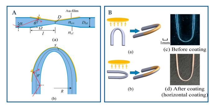
**Figure 4.** (**A**). Schematic diagram of the (**a**) straight and (**b**) U-shape of TPOF. Reprinted with permission from *Optik*, Copyright 2022, Elsevier [19]; (**B**). The schematic diagram of the coating results in the U-shaped probe based on POF (**a**–**d**). Reprinted with permission from *Optik*, Copyright 2022, Elsevier [19].
