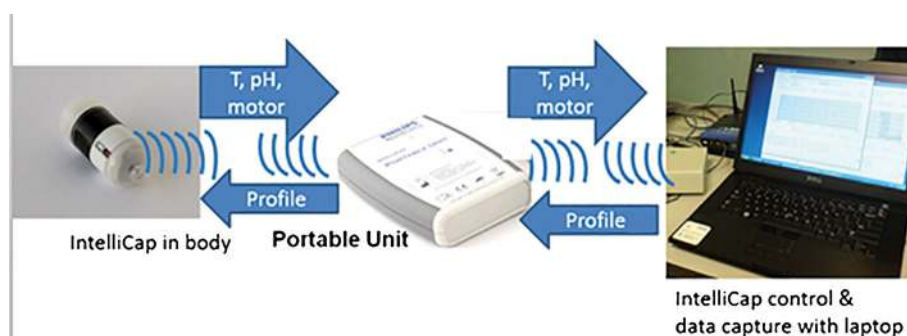
Fig. 2. IntelliCap® wireless data exchange scheme
