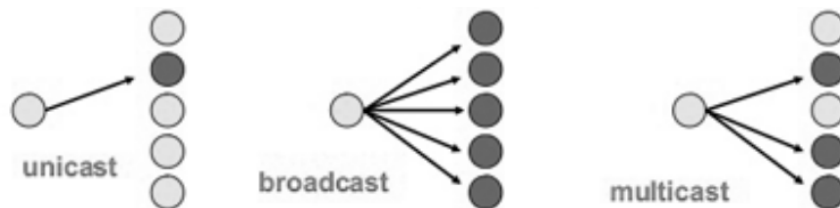
Figure III.2: Unicast, Multicast, Broadcast after Viraj Nevase 2016
