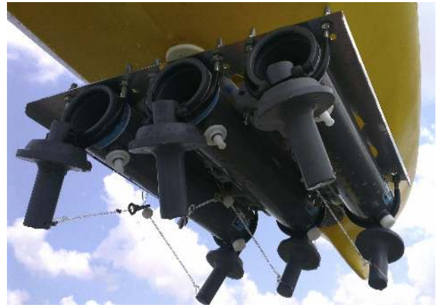
Fig. 3: Automated water sample collector.
