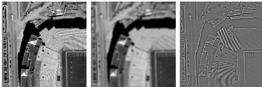
Fig. 5. One original image (left), main spatial trend extracted by 2D-SSA (middle) with parameters ( L_x=L_y=10 , 1 st component), and detailed structure extracted by 2D-SSA (right) with ( L_x=L_y=10 , 2 nd to 10 th components).
