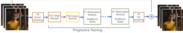
Figure 8: Illustration of the proposed framework by Boss-Gao. The team exploits cutting-edge deep neural architectures for the video quality mapping task, i.e PCD align module, TSA fusion module, residual blocks and RDN blocks. For progressive training, first, the PCD align module and the 1st Restoration module are trained together. Next, the TSA fusion module is plugged in and the existing parameters are used as initialization. Then, the new framework with TSA module is trained again. More restoration modules can be stacked to get a deeper framework, which can be trained to achieve better performance.
