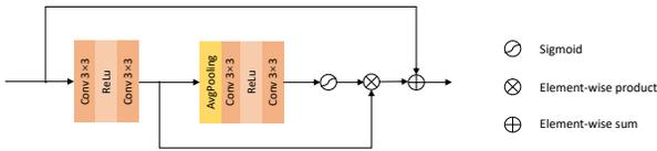
Figure 5: Residual Channel Attention Block
