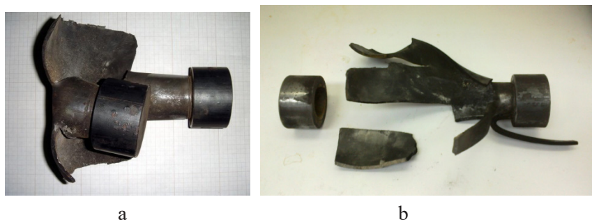
Figure 4. Results of the investigation on thermal ignition for (a) CompNTO and (b) cast TNT.
