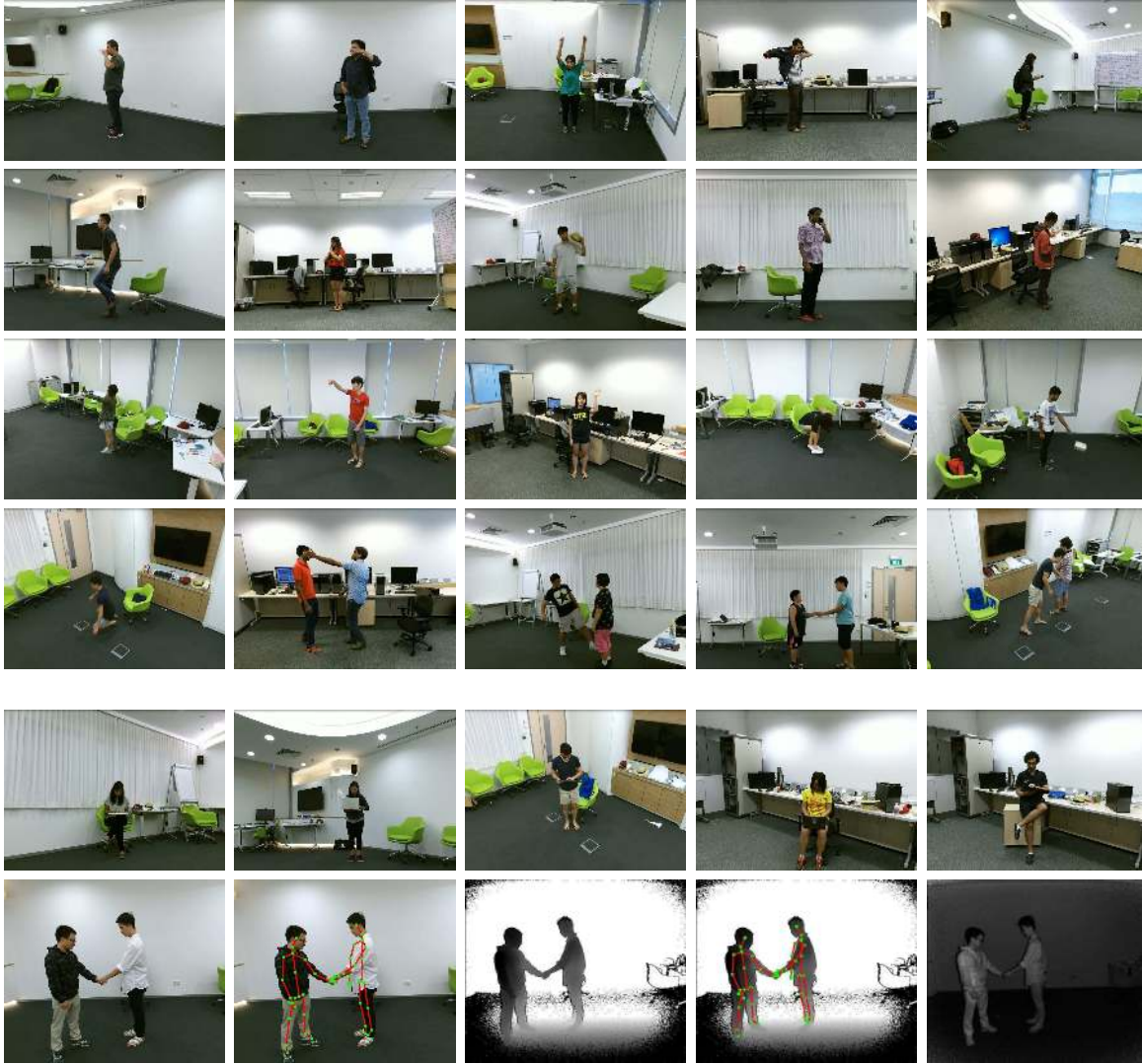
Figure 4. Sample frames of the NTU RGB+D dataset. First four rows show the variety in human subjects and camera views. Fifth row depicts the intra-class variation of the performances. The last row illustrates RGB, RGB+joins, depth, depth+joins, and IR modalities of a sample frame.
