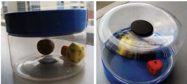
Figure 3: Container with dice (left) and revealing the RFID tag stuck to the bottom (right)
