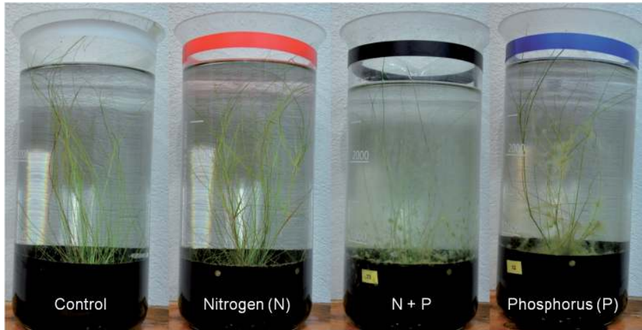
Fig. 9 Beakers representing the four treatment groups at the end of the growth experiment. The most obvious finding is the significantly (data not shown) higher periphyton abundance in the two P-treatment groups (paper III).
