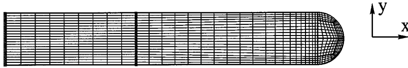
FIG. 7. Typical finite element mesh containing 748 elements. The locations of the periodic boundary conditions are shown by the thicker vertical lines.
