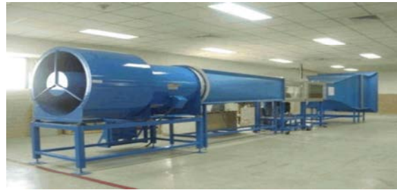
Fig. 6: Wind tunnel used for experiments
