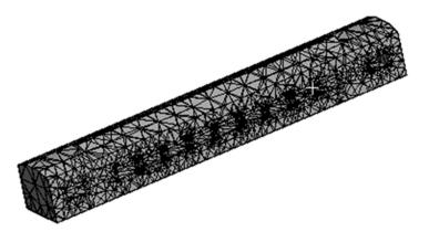
Figure 2. Mesh model of ICF passenger coach in ANSYS.
