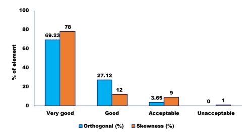
Figure 3. Mesh quality check using orthogonal and skewness quality.
