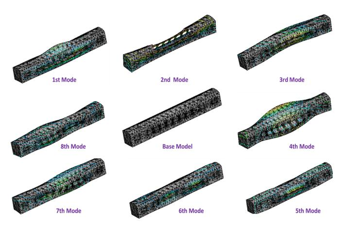
Figure 8. Modal frequency and mode shapes for passenger car body of ICF coach.
