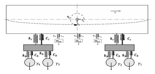
Figure 1. Schematic model of the passenger rail vehicle ICF coach.
