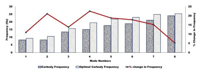
Figure 12. Effect of suspension parameter on the modal frequency of a CB.
