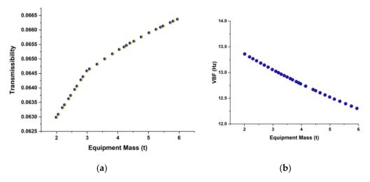
**Figure 11.** Elastic suspended equipment effect on CB mode due to equipment mass. (**a**) Transmissibility, (**b**) VBF.
