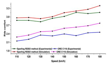
the experimentally measured results. The variation in the ride index is mainly due to the elements not considered to reduce the complexity of the mathematical model.
