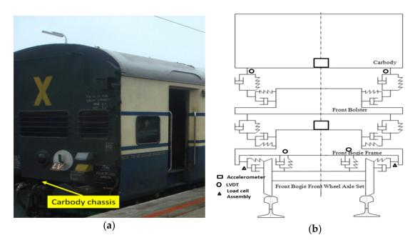
Figure 6. Field test line diagram of ICF coach. (a) ICF coach; (b) sensor location.
