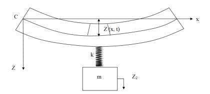
Figure 5. Model of the DVA applied on a flexible beam [13].
