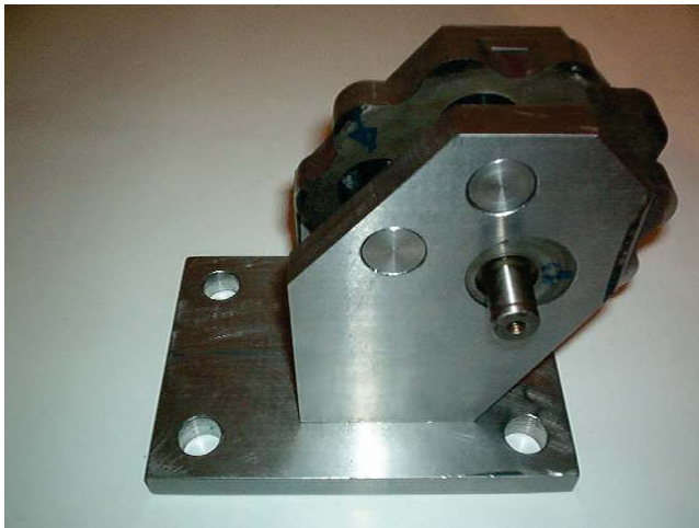
Figure 7 Physical model of the tool for investigation of the stress state of the cycloid disc
