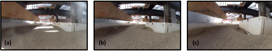
Figure 3.8. Snapshot from video camera located near the northeast corner of the aligned foundation during Test Day 2 after the end of; (a) motion 4 (Pacoima Dam at 80%), (b) motion 5 (Takatori at 50%), and (c) motion 6 (Takatori at 100%).
