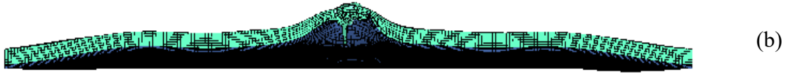
Fig 9 Comparison of (a) experimental and (b) numerical results with the rubber on the back face at the impact velocity of 144 m/s
