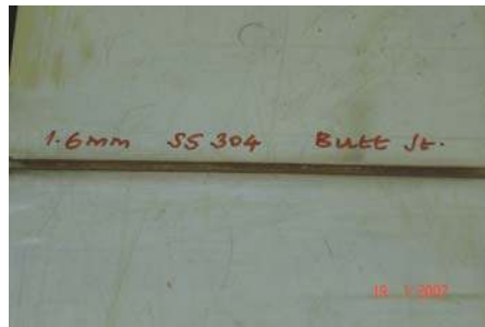
Figure 6: Butt-joint sample test coupon after laser welding showing a smooth bead finish.
