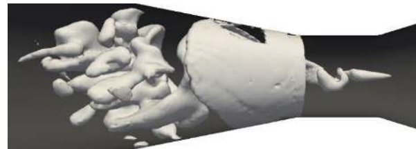
Figure 21 Helical vortex breakdown captured using the CFD
