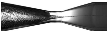
Figure 18 Cavitating vortex filament downstream the SG
