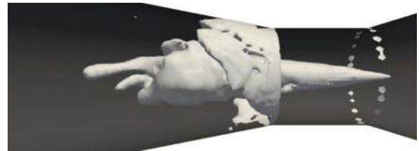
Figure 20 Cavitating vortex captured using the CFD
