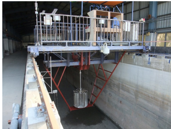
Figure 6. Towing tank experimental platform.
