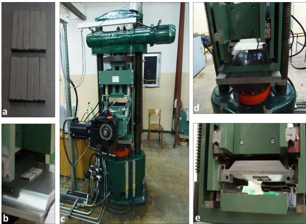
Fig. 6—Test stand for incremental forming process: (a) anvils, (b) anvils put in a test stand, (c) hydraulic press, (d) work station zoomed view, and (e) work station with anvils prepared for IF process.
