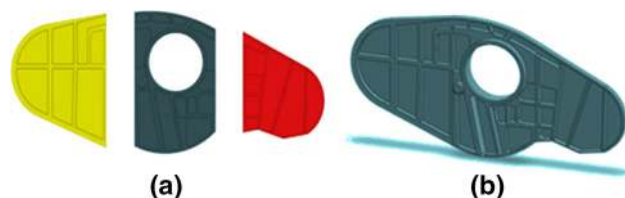
Fig. 1—Example of a part made from (a) many smaller elements in a conventional approach, (b) one piece of material—integral element.
