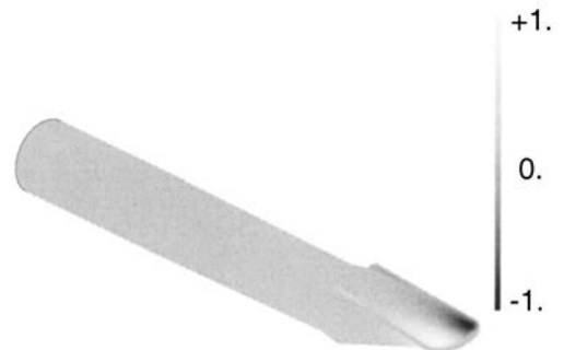
FIG. 6. Computed eigenmode at 4119 Hz in a mixed solid-air situation: acoustic pressure inside the mouthpiece and barrel.
