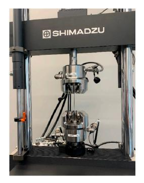
Figure 2. Fatigue loading machine (Shimadzu, EHF-LV020K1A).
