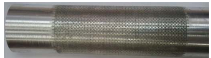
Fig. 4. Circles engraved on the tube.
