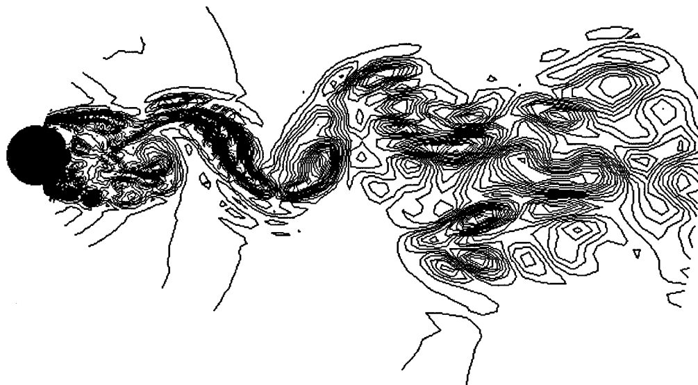
Figure 57: Re = 3,900 ; Instantaneous spanwise vorticity contours in the first 10 diameters of the vertical plane z = 0 (seventh-order scheme)
