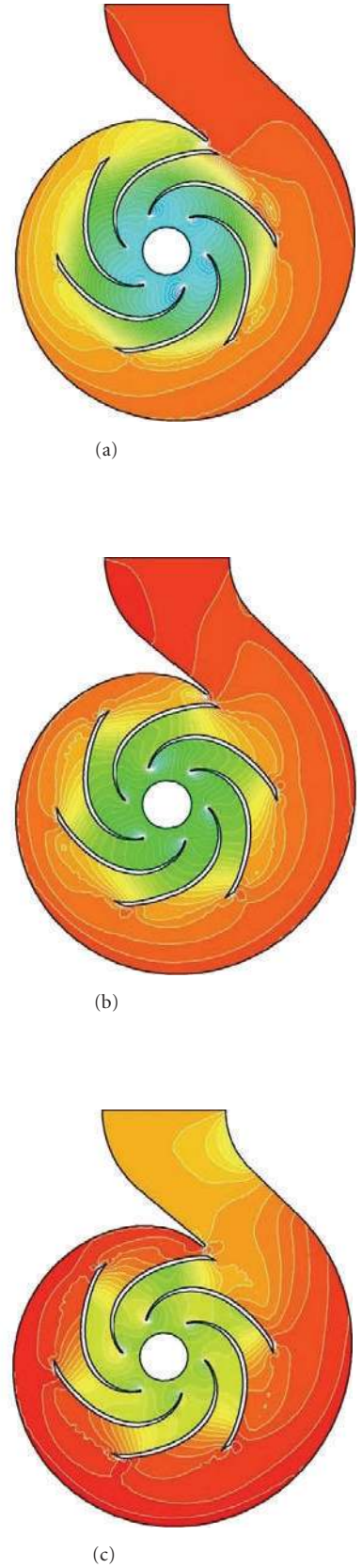
FIGURE 8: Pressure distribution inside impeller and volute. (a) Off-design point, Q = 0.43 Q_{design} . (b) Design point, Q_{design} . (c) Off-design point, Q = 1.45 Q_{design} .
