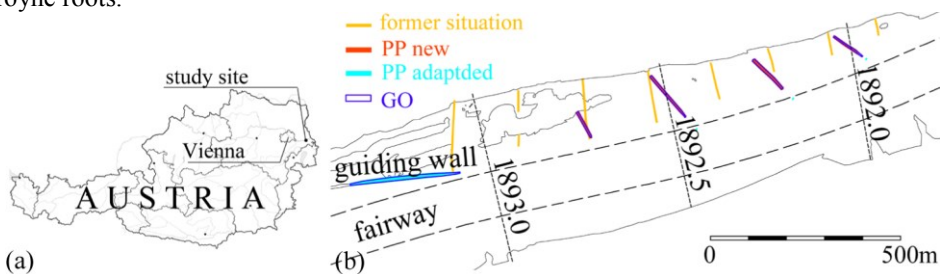
Fig 1. (a) Overview. (b) Sketch of the study site including the former groyne layout (2007), the adaptations during the PP (2008/2009) and the groyne layout optimisation GO (2016). Flow direction is from left to right.
