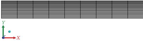
FIGURE 2: Mesh layout of present geometry, axisymmetric about X-axis.
