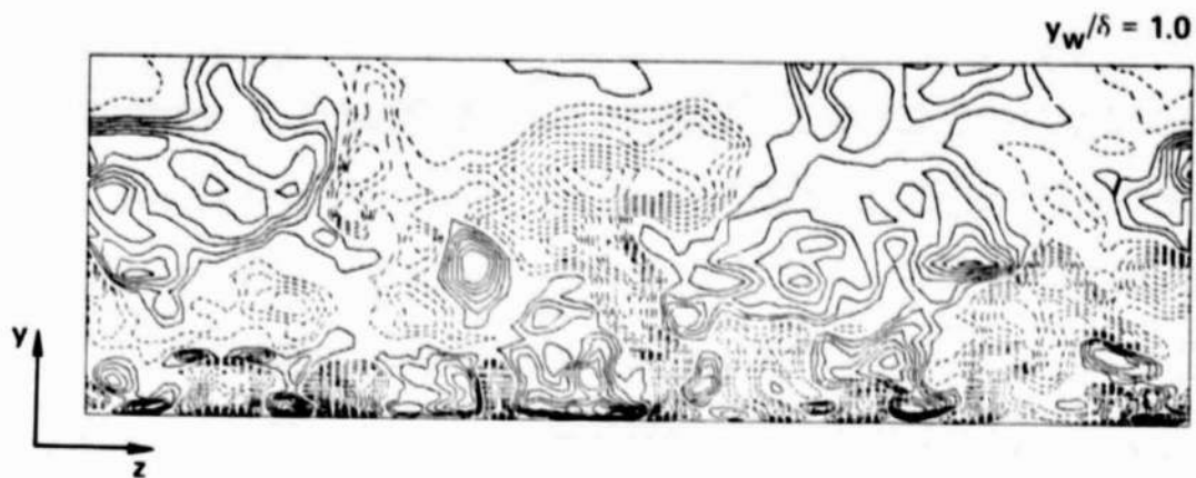
Fig. 25. Contours of \bar{u} in the y - z plane at x = 0 . (Only the lower half of the channel is shown.)
