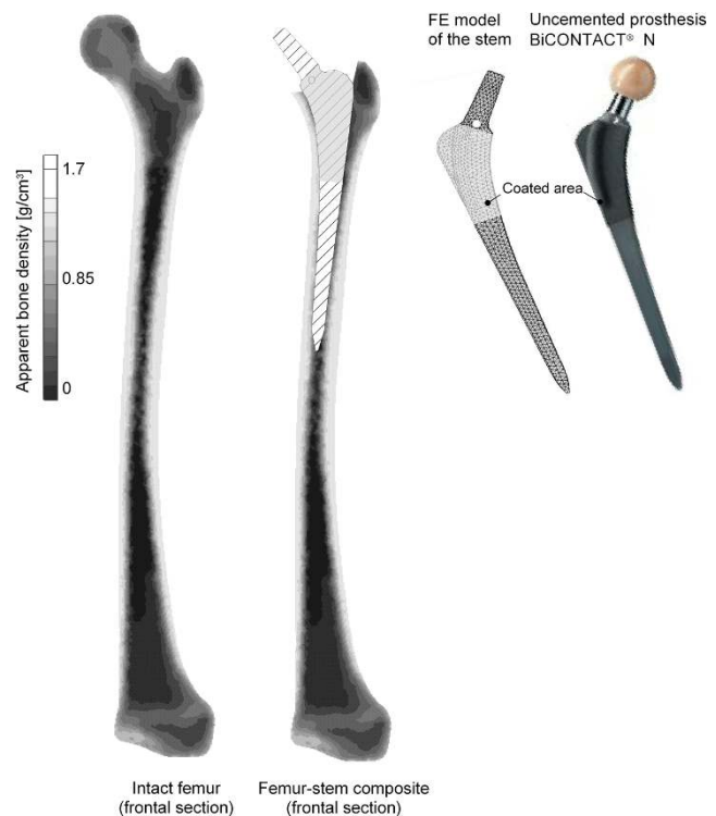
Figure 1 FE model of the intact femur (left), the composite (middle) and the stem used (right). This figure shows on the left side the distribution of the ABD in the frontal section of the intact femur. In the middle the frontal section of the composite femur-stem is illustrated. On the right side an image and the FE model of the conventional uncemented BiCONTACT® N prosthesis are presented.
