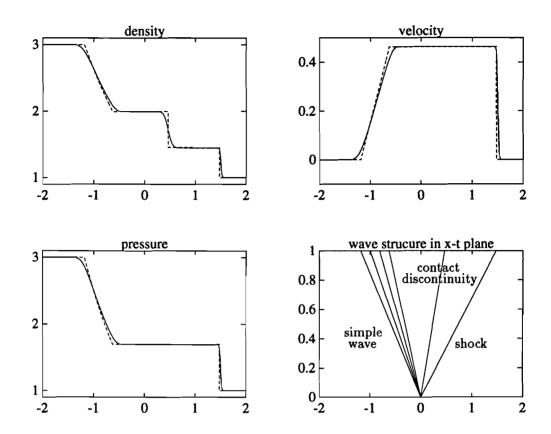
Figure 3: Numerical solution (solid line) computed with Osher's method (with  $\tau = 0.1$ ) and exact solution (dashed line) at time t = 1 of a shock tube problem for the one-dimensional Euler equations (2.7) with initial conditions p(x,0) = 3,  $\rho(x,0) = 3$ , u(x,0) = 0 if x < 0 and p(x,0) = 1,  $\rho(x,0) = 1$ , u(x,0) = 0 if x > 0.
