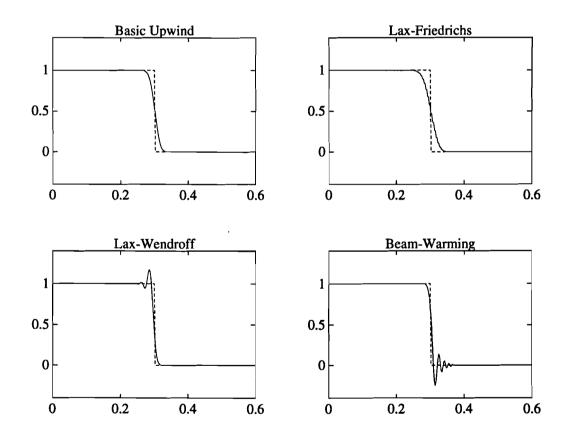
Figure 2: Numerical solution (solid line) and exact solution (dashed line) of (4.11) at t = 0.3 with  $a = 1, \Delta t = 0.002, \sigma = 0.8$  and the initial condition u(x, 0) = 1 if x < 0 and u(x, 0) = 0 if x > 0.
