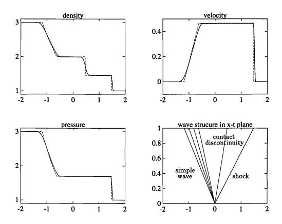
Figure 4: Numerical solution (solid line) computed with Roe's method (with  $\tau=0.1$ ) and exact solution (dashed line) at time t=1 of a shock tube problem for the one-dimensional Euler equations (2.7) with initial conditions p(x,0)=3,  $\rho(x,0)=3$ , u(x,0)=0 if x<0 and p(x,0)=1,  $\rho(x,0)=1$ , u(x,0)=0 if x>0.
