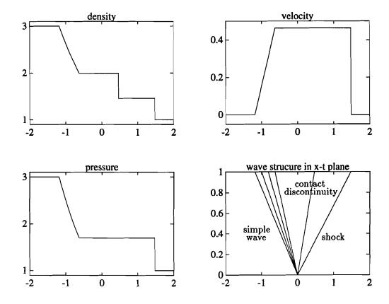
Figure 1: Solution at time t=1 of a shock tube problem for the one-dimensional Euler equations (2.7) with initial conditions p(x,0)=3,  $\rho(x,0)=3$ , u(x,0)=0 if x<0 and p(x,0)=1,  $\rho(x,0)=1$ , u(x,0)=0 if x>0.
