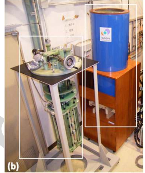
Fig. 2. (a) Schematic of the experimental system for the measurement of dynamic loss in an HTS-coated conductor, and (b) picture of the system with an ac magnet and a sample holder (left), and a cryogenic container (right).
