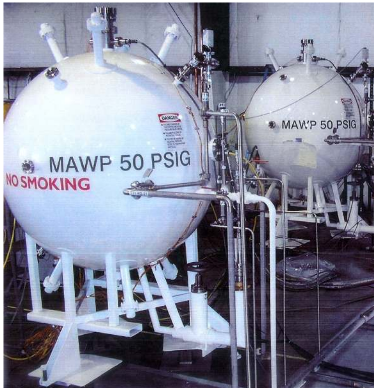
Figure 2. Two 1,000-L demonstration tanks for measuring boiloff of liquid hydrogen and nitrogen using glass bubbles and perlite insulation.
