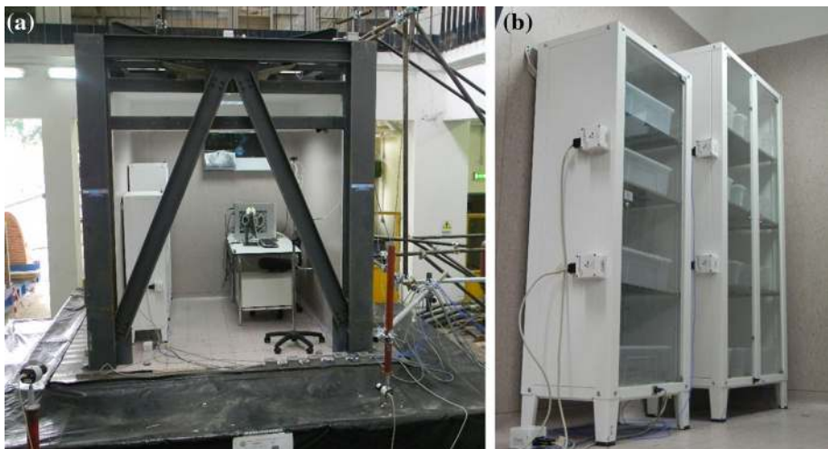
Fig. 1 a Global view on the tested hospital examination room and b close-up view on the two cabinets
