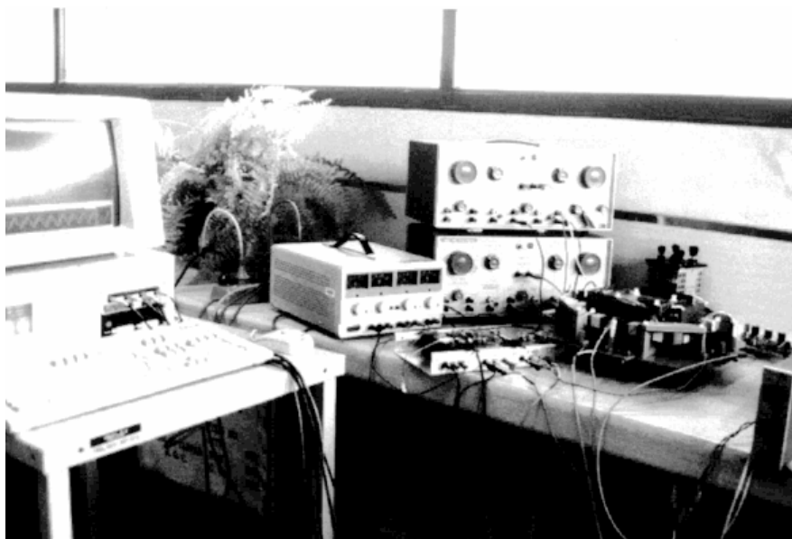
Fig.5-1 A photograph of the rotational core loss measuring system developed at UTS
