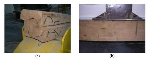
Figure 6. Failure modes: (a) unreinforced timber beam; (b) reinforced beam.
