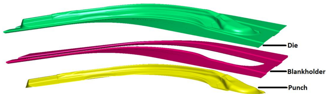
Figure 3. The tool geometry in the PAM-Stamp 2G software.
