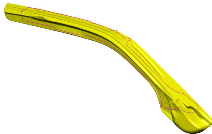
Figure 5. The trimming curve on the punch.
