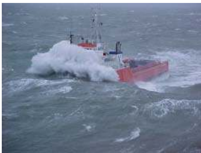
Figure 1.1: Example of green water load on a small vessel.
