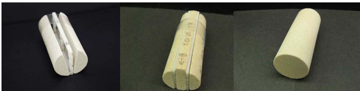
Figure 11 – Three different core configurations for different experiments. The single- and double-fracture designs were used during exchange studies, while non-fractured samples were used for resistivity, depressurization and additional exchange studies.
