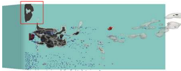
Figure 14. Overestimation of cavitation inception on the lower wall by the Eulerian model (on the left of the cylinder) compared with the hybrid model prediction with no spurious cavity (on the right of the cylinder).
