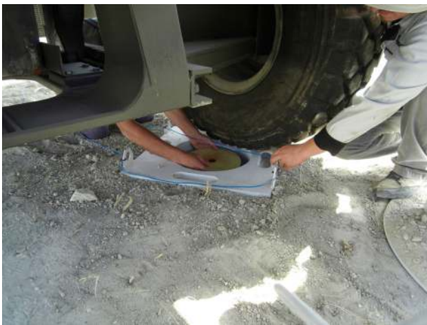
Fig. 19 Placement of the land mine in the steel pot under the front left tire
