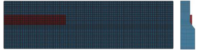
FIGURE 9: The front view and side view of calculation model of blasting excavation of rock-anchored beam (unit: m).
