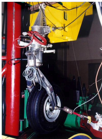
Figure 3: A gear landing during the test
