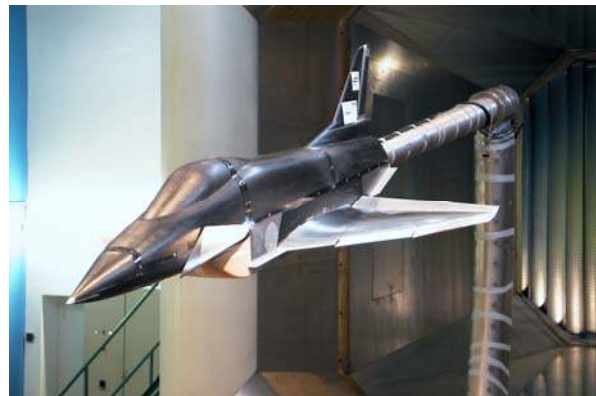
Figure 4: X-31-Remote-Control-Model in the DNW-NWB Braunschweig.
