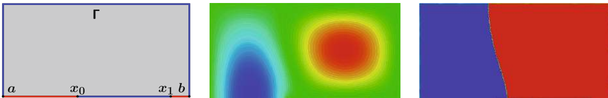
FIGURE 16. Eigenmodes for the Neumann-Dirichlet-Neumann problem on the half-square. Left: the domain; center: the second eigenfunction; right: the associated nodal domains.
