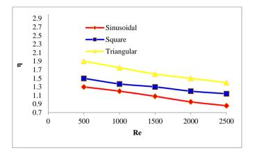
Figure 6. The variation of the thermal-hydrodynamics performance for various Reynolds number for all cases
