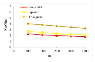
Figure 4. The variation of the thermal enhancement ratio for various Reynolds number for all cases
