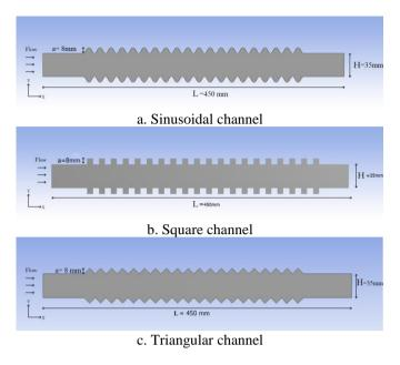
Figure 1. Schematic diagram of the corrugated channel
