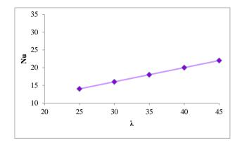
Figure 7. Effect of the corrugated angle on Nusselt number at Re=2500
