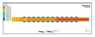
Figure 14. Velocity contour for 30° degree angled pipe, 2500 Reynolds number
