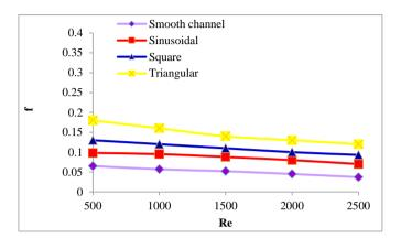
Figure 5. The variation of the friction factor for various Reynolds number for all cases
