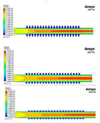
**Figure 11.** Velocity contour (sinusoidal, square and triangular) channels for Reynolds number Re=500
