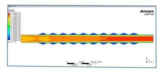
Figure 13. Velocity contour for 25° degree angled pipe, 2500 Reynolds number
