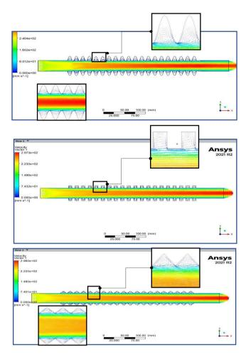
Figure 12. Velocity vector (sinusoidal, square and triangular) channels for Reynolds number 500
