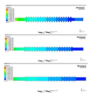
Figure 10. The pressure in (sinusoidal, square and triangular) channels for Reynolds number 500
